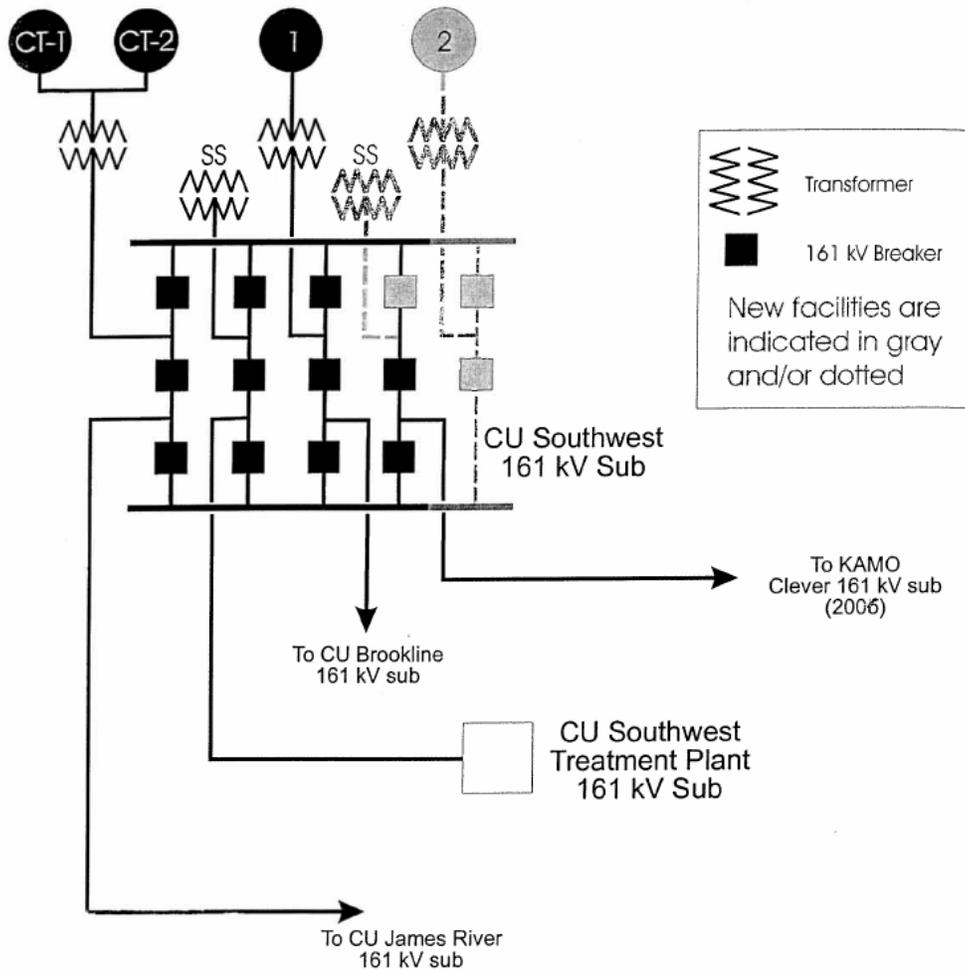
Figure 1. Interconnection Plan for GEN-2006-019 to the 161 kV System
